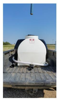
Gap between tank and filler pipe
