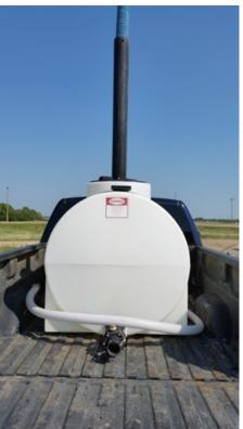
Tank with extension pipe made from ABS or PVC pipe
